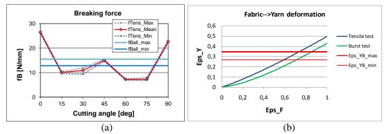
Figure 10: Specific breaking force versus cutting angle (a) and the relationship between the strains of the fabric and its yarns (b) in cases of tensile and burst tests
