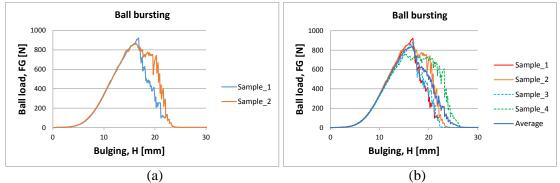
Figure 9: Typical load-deformation relationships (a) and the average of four measurements (b)
