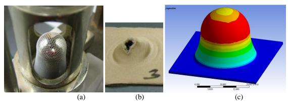
Figure 2: Concave deformed shape of material of large deformability (a) as well as shape of rupture (b) and stress results of FEM simulation performed for foam laminated knitted fabric (c)
