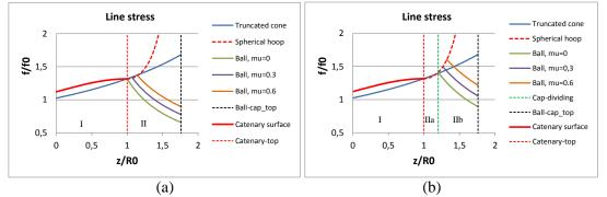
Figure 6: Normalized meridian stress along the axial section of the deformed sample without (a) and with (b) free hoop (IIa) on the spherical cap ( $mu=\mu$ )
