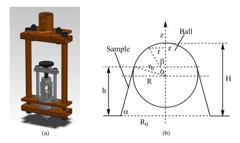
Figure 1: Ball bursting apparatus (a) and the classic scheme of bursting (b)
