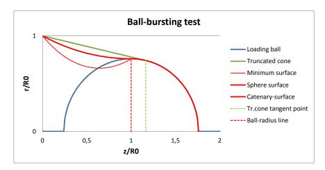
Figure 4: Schematic normalized plane section of the middle surface of the deformed specimen along the axis of rotation (H/R<sub>0</sub>=1.76) in cases of different approaches (min. surf:  $c_0=1$ ,  $c_2=c_1R_0=1.316$ ; catenary:  $c_0=0.589$ ,  $c_2=c_1R_0=0.775$ )
