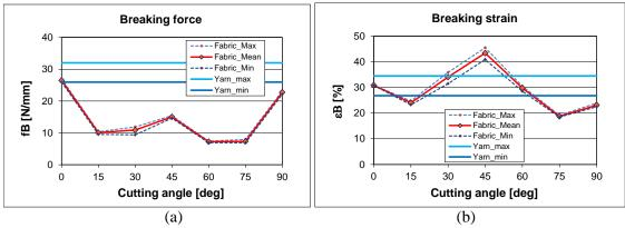
Figure 7: Measured values of the specific tensile breaking force (a) and the breaking strain (b) versus cutting angle
