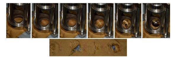
Figure 8: Deformation process of the woven fabric sample during the ball burst test and the shape of the split holes
