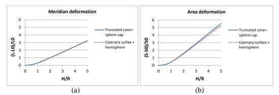
Figure 5: Linear meridian (a) and area (b) strain as a function of the normalized bulging
